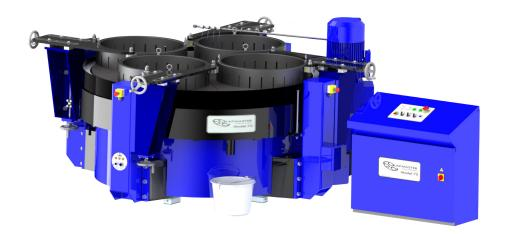
The Lapmaster Wolters model 72 is equipped with a 1829mm diameter lap plate. This is manufactured from Grade 300 grey cast iron to ISO 185(2005). It consists of individual segments bolted to a support plate.
